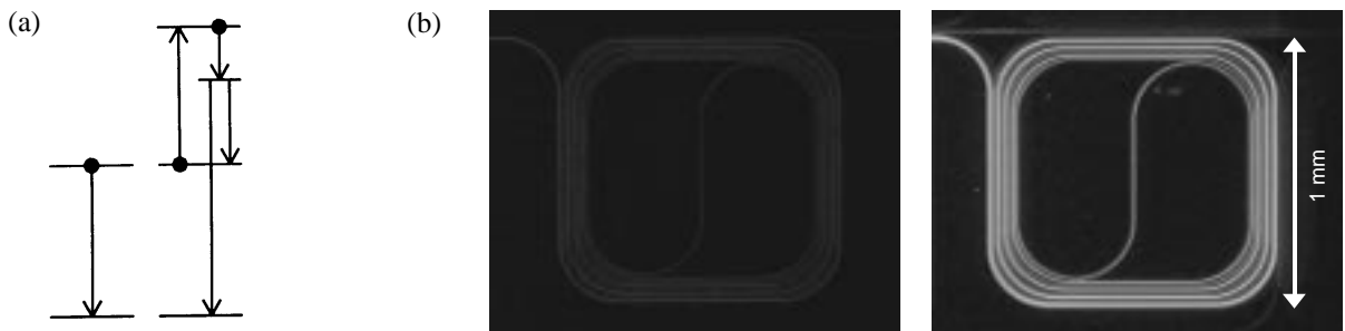
Fig. 3 (a) Schematic of cooperative upconversion in \text{Er}^{3+} . (b) Optical images of two \text{Al}_2\text{O}_3 waveguides doped with Er to the same concentration (0.3 at.%) pumped at 1.48 \mu\text{m} . Left: doped by ion implantation, Right: fabricated by \text{Al}_2\text{O}_3/\text{Er}_2\text{O}_3 co-sputtering. The green emission from the waveguides is represented in white. From Kik et al. , Ref. 8.
