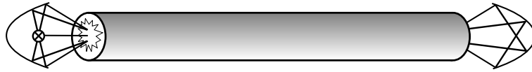
Figure 6.5: Prism light guide for high illumination intensities. The light is reflected inside the tube. The sawtooth prisms at the walls reflect up to 99 % of the light and couple out the rest. Illumination lengths of 20 m and more are obtainable.
